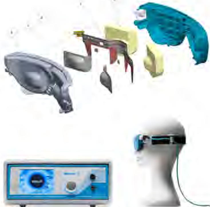
FIGURE 1. Rexion-Eye device. Top panel: An exploded view of the Rexion-Eye goggle electrode, with electronic board (1), temperature sensors (2), active electrodes (3), external plastic shell (4), internal rubber layer (5), internal sponge filling (6). Bottom panel: The Rexion-Eye device, with electrical generator (left side) and goggle electrode (right side).
