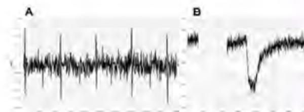
Fig. 6 Change in membrane potential as monitored by fluorescence of Di-8-ANEPPS. A) Fast changes related to single pulse stimulation, likely corresponding to action potential. B) Long lasting change due to application of high frequency low power electrical field. On the abscissa a small division corresponds to 40 ms in A and 100 ms in B
