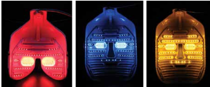
Figure 2. The inside of the Epi-C Plus device's light modulation mask is embedded with LED lights.
