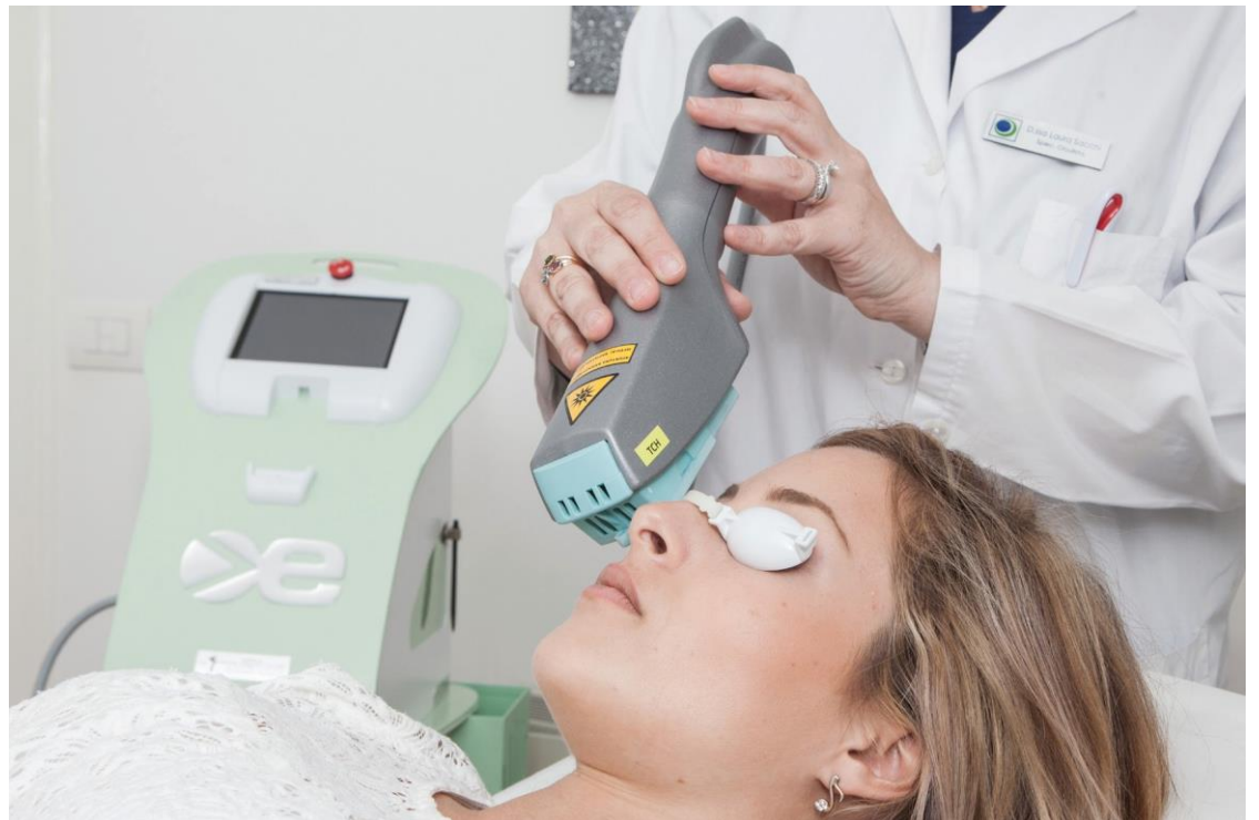
Fig. 1 Handpiece for the application of the pulsed light of the Eye-Light instrument
